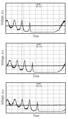
This data series was taken with a Model 6428 Vidia-Swept tunable laser, and illustrates the 60-pm response shift of a fiber-Bragg grating over 57.6° to 0° C. The scan speed is 1 nm/sec and the trigger setting is 1563.40 nm.
